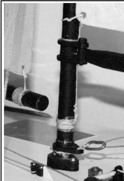
String Rings used to adjust the jib outhaul and mainsail downhaul
