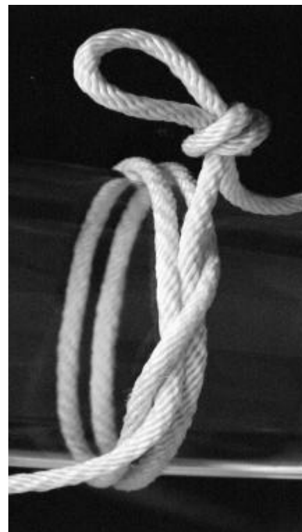
String Rings used to adjust the jib outhaul and mainsail downhaul
