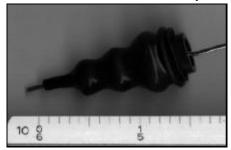
mechanically rugged. It is best to have the female portion on the battery lead. There is always the chance that the exposed pins of the male portion could be shorted by contact with something conductive.
