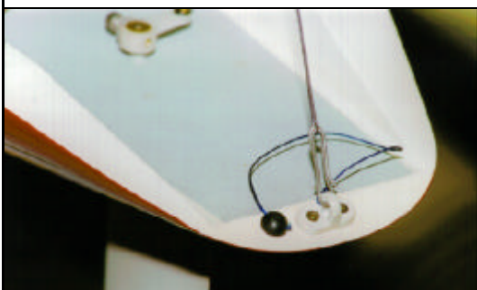
The photo illustrates an alternate location for the necessary drain hole plug. The other location is on deck at the extreme tip of the
