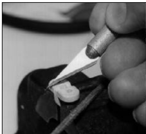
Groove the eyelet to recess the line
