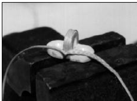
Reinforce the eye with wraps of line
