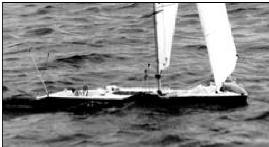
Buttons Padin's "Gonzo" on a High Speed Run Note the bow wave over the bow and on deck and a wave boarding amidships. The bow is pressed deep into the water. Submarine and broach is imminent.
